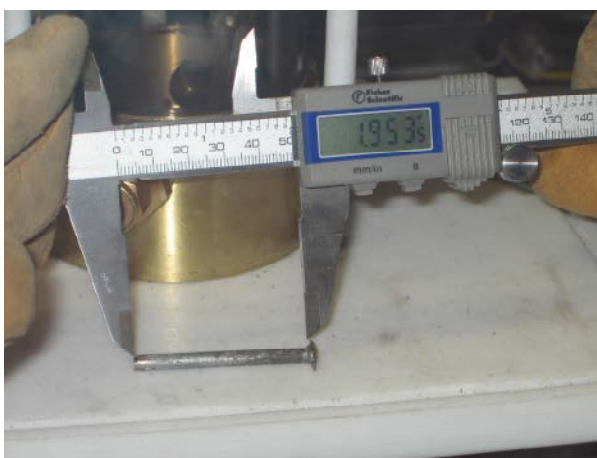
Figure 2.13: MA-bearing fuel alloys for AFC-2 irradiation test [36]
