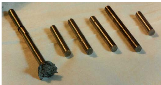
Figure 2.13: MA-bearing fuel alloys for AFC-2 irradiation test [36]
