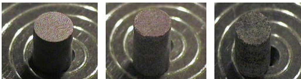
Figure 5.11: Visual appearance (from left) of CAMIX 1, CAMIX 2 and COCHIX 3 pellets
