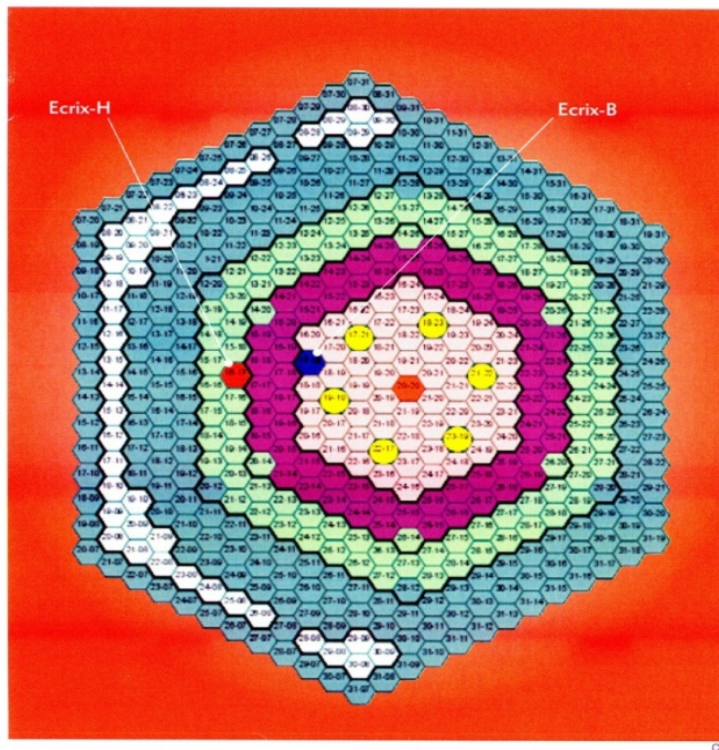
Figure 5.22: Location of the ECRIX pin in Phénix core [18]
