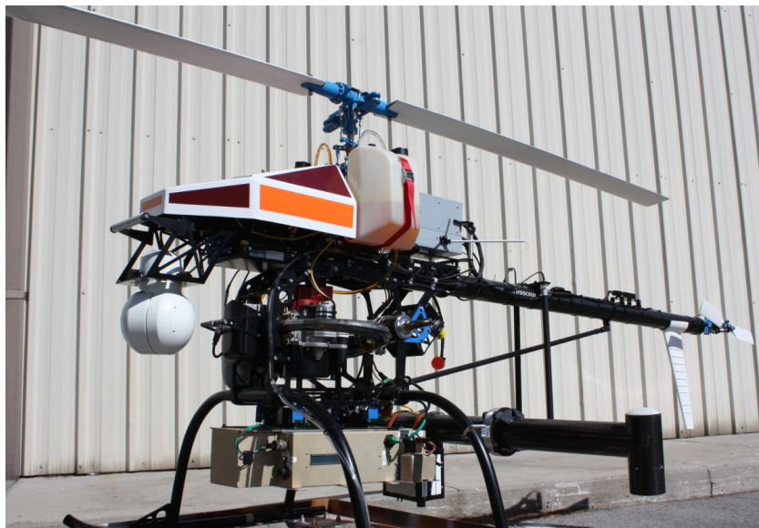
Figure 6.25: Sensor system components installed on an Aeroscout B1-100 helicopter
