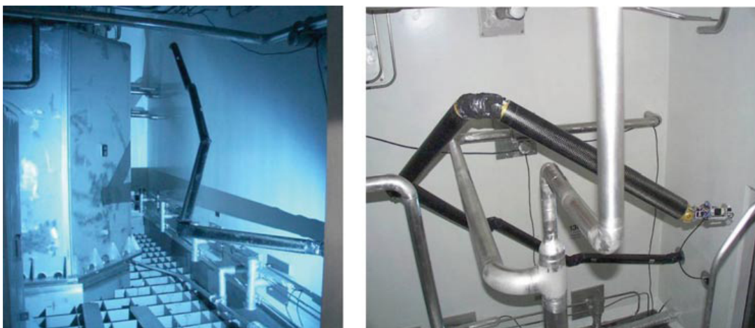
Figure 6.20: Introduction in the cell (left) and pipe avoidance during inspection (right)
