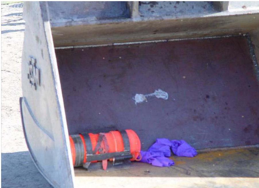
Figure 5.12: Steel plate welded in bucket creates uniform soil thickness for sodium iodide monitoring
