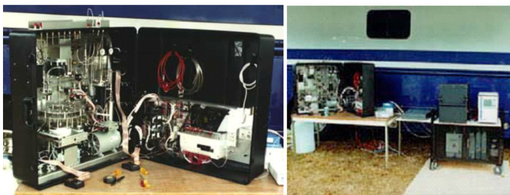
Figure 6.28: FDTAS-tritium analysis system in surface and groundwater in near real time
