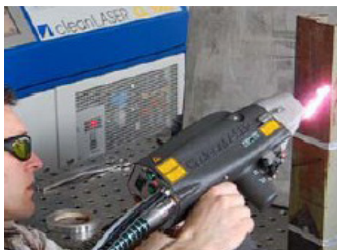
Figure 4.2: OSH 80 laser paint stripper
