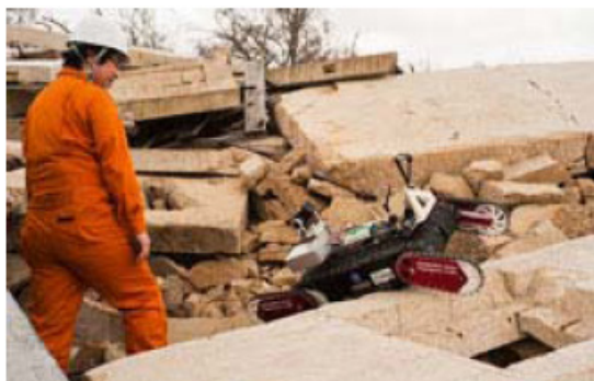
Figure 4.9: Quince being tested at disaster city rubble pile the week before the Fukushima Daiichi NPP accident
