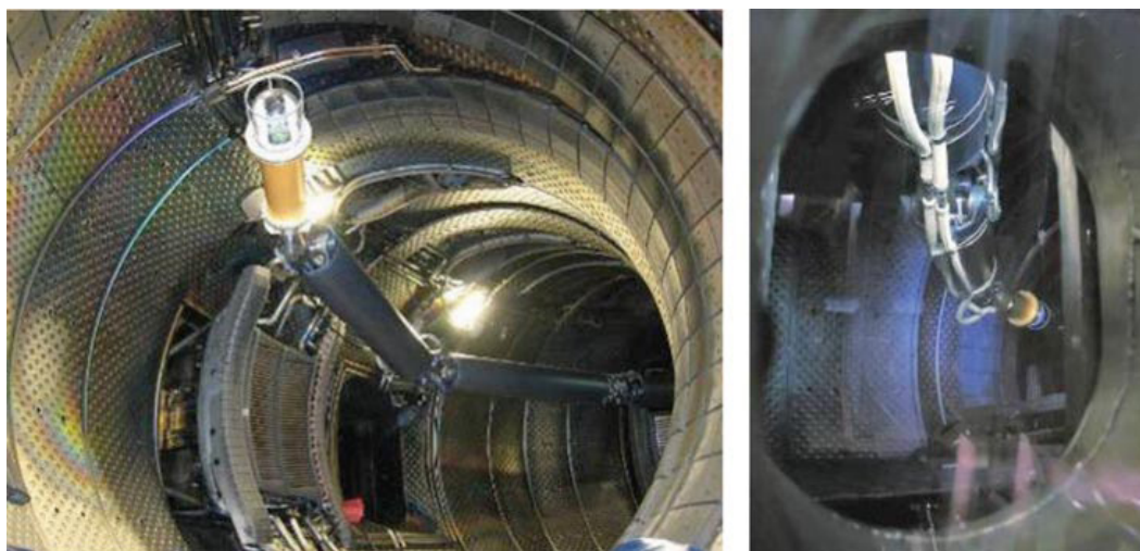
Figure 6.22: AIA robot inspection in Tore Supra Tokamak during air operation (left) and window view during operation under vacuum and at temperature (right)
