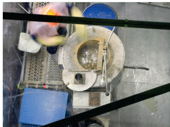
Figure 4.7. On-site melting of lead using furnaces
