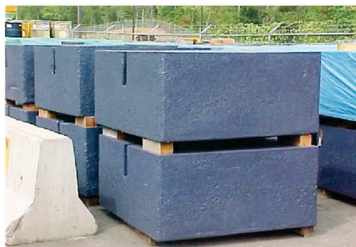
Figure 4.1. Shield blocks manufactured at EnergySolutions' Bear Creek Facility
