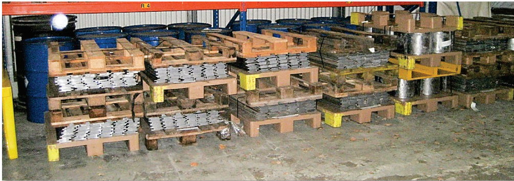
Figure 4.6. Lead-filled shielding blocks for constructing movable shielding walls
