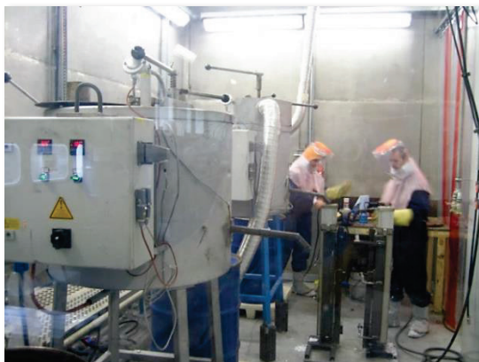
Figure 4.7. On-site melting of lead using furnaces
