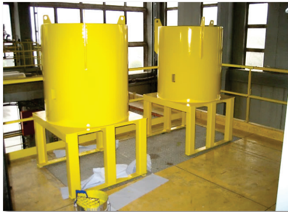
Figure 4.5. Shielding containers for 400-litre drums
