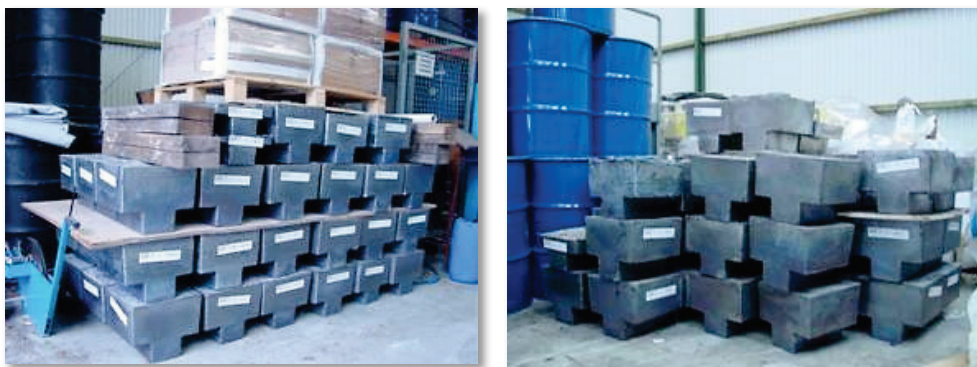
Figure 4.4. Unconditionally cleared lead ingots from on-site melting at the BR3 NPP
