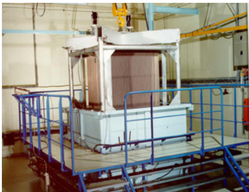
Figure 1. Apparatus B – general view of fuel rods array setting up in the core tank
