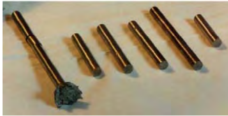
Figure 7: Cast fuel rods
