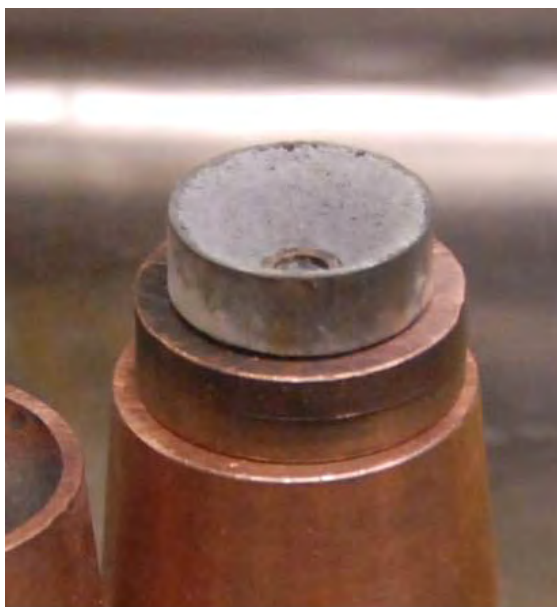
Figure 1: A new copper hearth for drop casting
