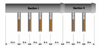
"...simulate part of a future KBS-3 repository to the extent possible with respect to geometry, design, materials, construction and rock environment except that radioactive waste is simulated by electrical heaters, and to test and demonstrate the integrated function of the repository components."
