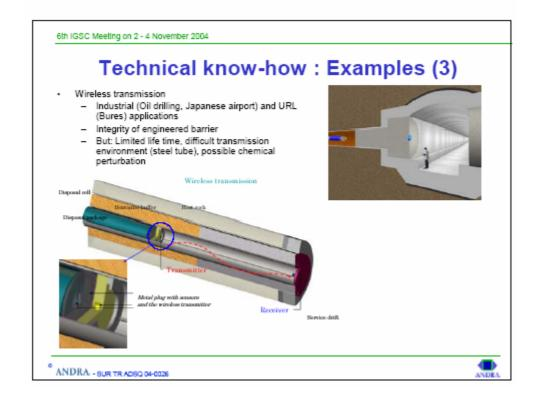
Example: Monitoring in a B-type waste tunnel
