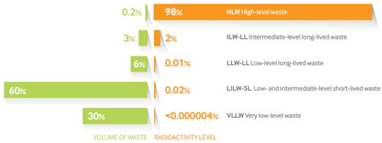
► BREAKDOWN BY VOLUME AND RADIOACTIVITY LEVEL OF RADIOACTIVE WASTE PRESENT AT THE END OF 2013
