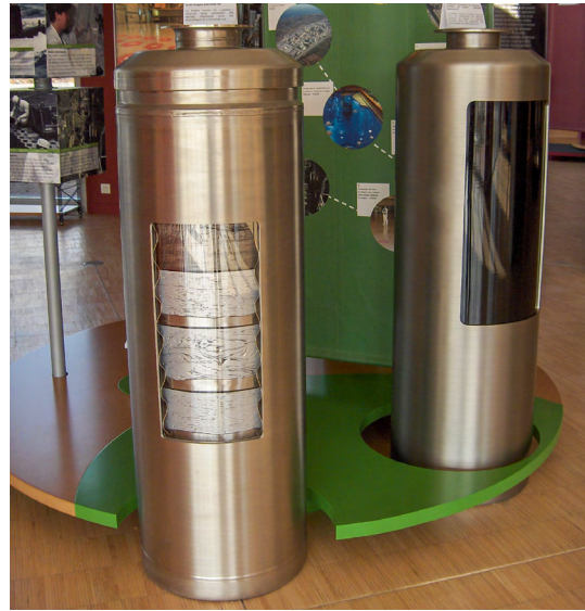
Standard containers for high-level (right) and medium-level (left) waste at the Meuse and Haute-Marne underground research laboratory in Bure.
