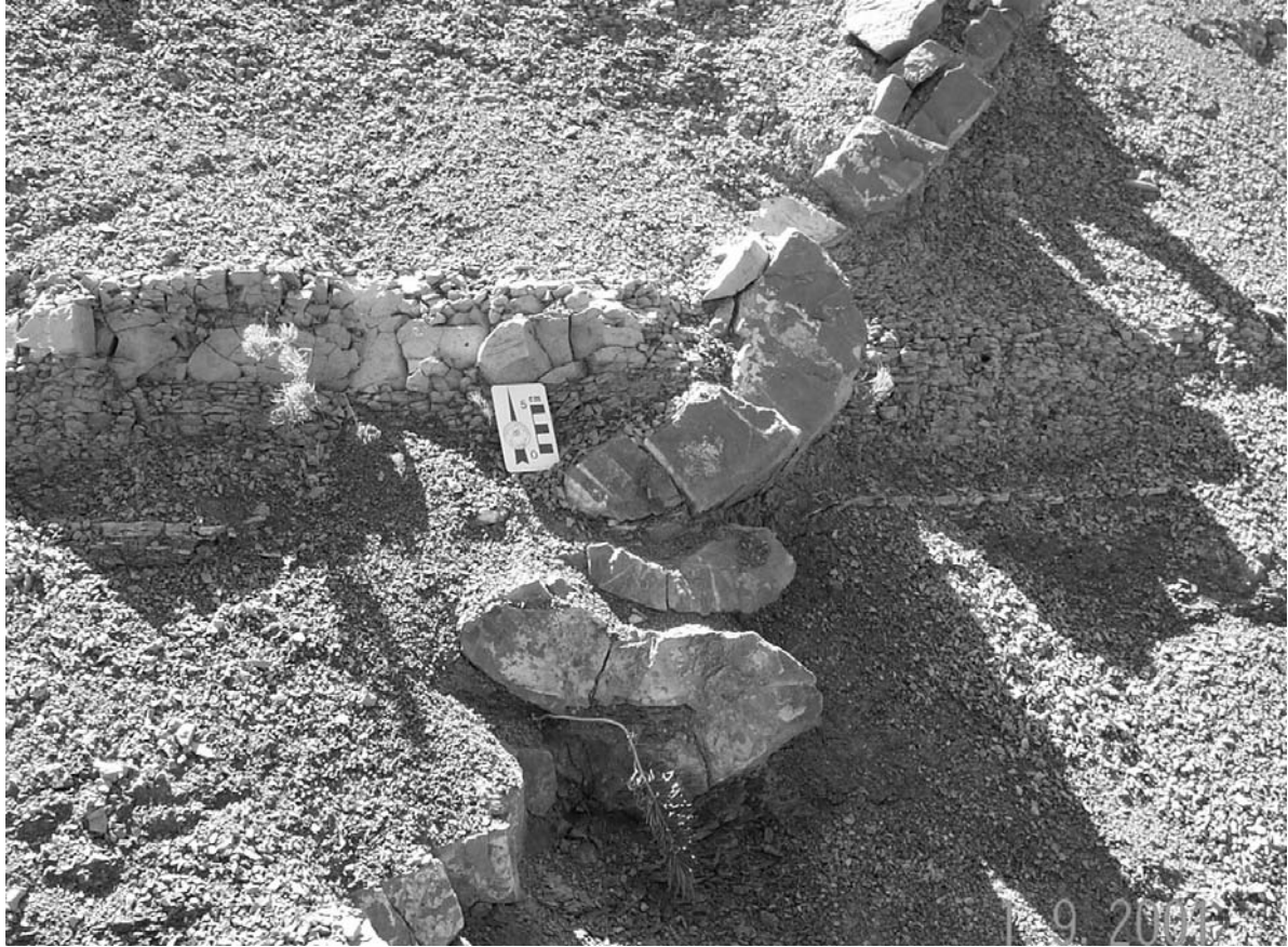
Figure 4. Compacted dyke in the aptian marls of Bevons The post-injection compaction rate ( \tau = h_0/h ) may be directly measured
