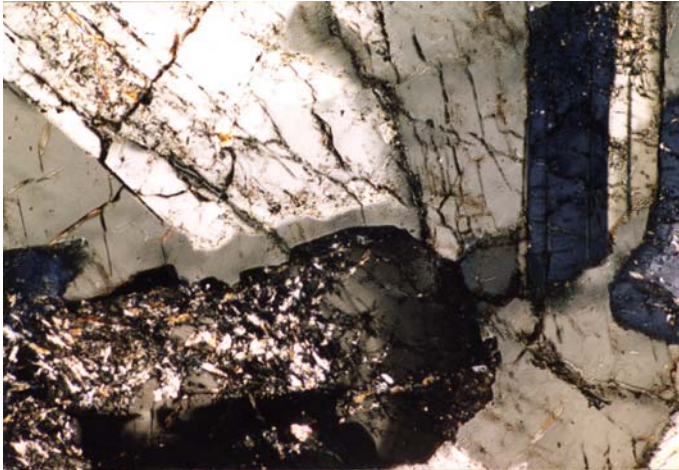
Figure 1. Impregnation of weakly altered feldspars from the Kurihashi granodiorite, Kamaishi Mine, Japan (from [1]).
