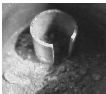
Figure 2.3-10: 83 MWd/kgU UO 2 fuel fragments that moved out of a pre-cut cladding after a 1 200°C heating test.
