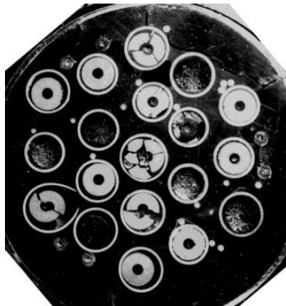
Figure 2.4-3: Cross-cut of test assembly of MIR/LOCA-50 test at elevation 830 mm from bottom [2.4-3]
