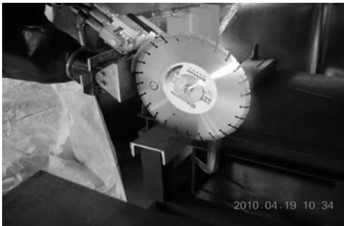
Figure 73: Remote grip and transfer device - Handling tests using test pieces
