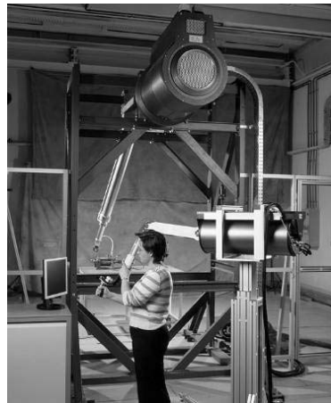
Figure 7: Re-engineering of an existing master-slave manipulator with electrical power and remote control
