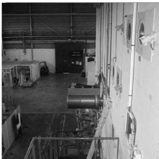
Motor box replacing the conventional master arm and its counterweights
