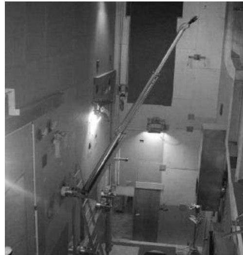
Slave arm inside the hot cell in "ceiling configuration"
