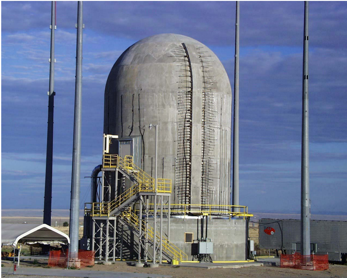
Figure 2.4 Completed PCCV Model
