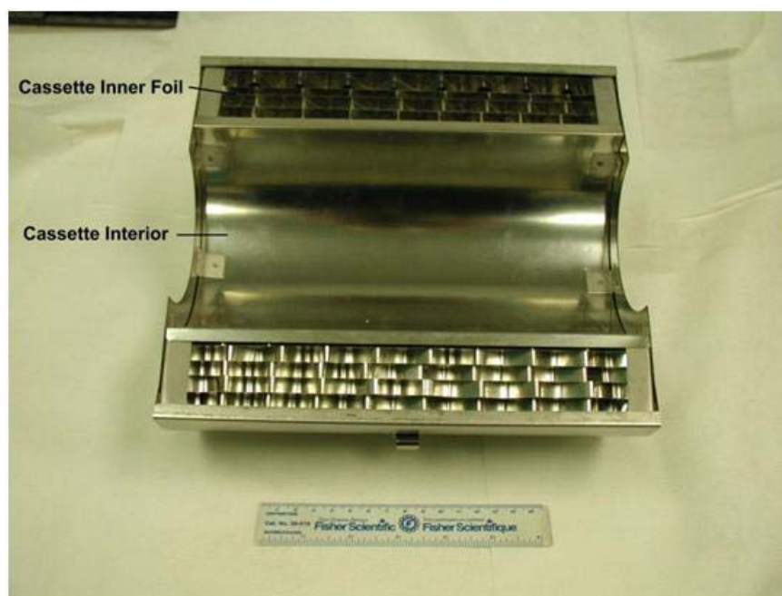
Figure 4. Photograph of an Inverted RMI Cassette showing where Type B (Cassette Interior) and Type C (Cassette Inner Foil) sample discs were taken
