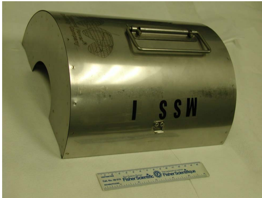
Figure 5. Photograph of RMI Cassette showing where Type D (Cassette Exterior) sample discs were taken
