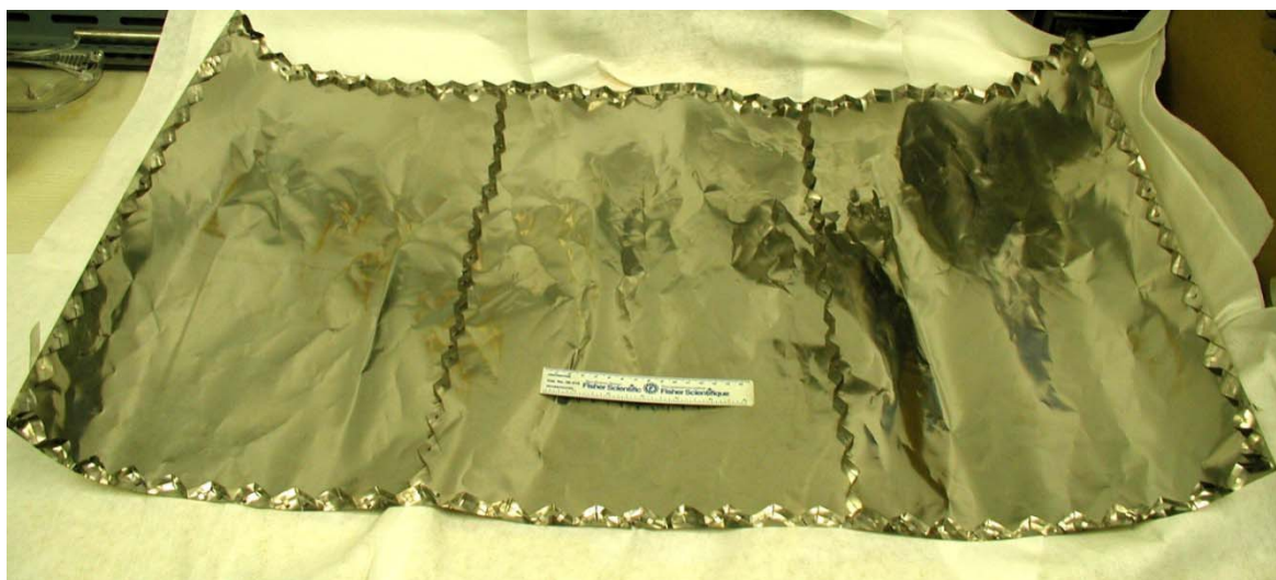
Figure 3. Photograph of RMI Type A from which a 1.27 cm diameter discs were punched
