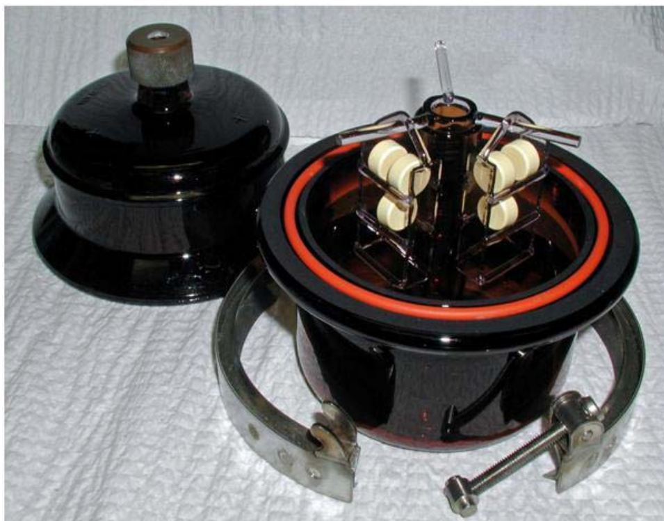
Figure 11. Irradiation Vessel (Post-irradiation, with Coupons and Holders)
