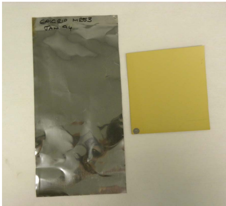
Figure 6. Photograph of EPIGRIP M253 Coated Metal (Base Metal for 1994 sample and Painted Surface of 1998 Sample Shown).
