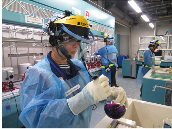
Worker analysing radioactivity concentration and water quality of samples collected at and around the Fukushima Daiichi Nuclear Power Plant. A work support device called “smart glasses” is worn to improve the productivity and quality of data entry and confirmation. Source: TEPCO Holdings
