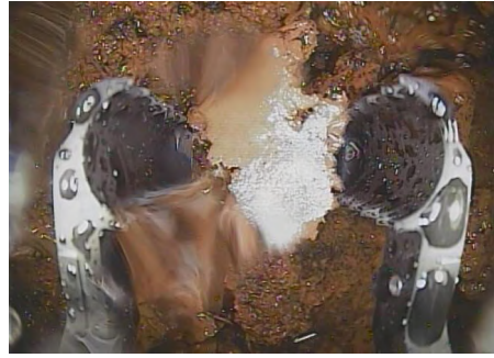
Fuel debris inside the primary containment vessel in the Unit 2 reactor building of the Fukushima Daiichi Nuclear Power Plant. (Fuel debris is a substance that has cooled and re-solidified while being mixed with various materials after the fuel in the reactor melted as a result of the accident.) The debris can be removed with a robot replicating the grip and movement of fingers. Source: TEPCO Holdings
