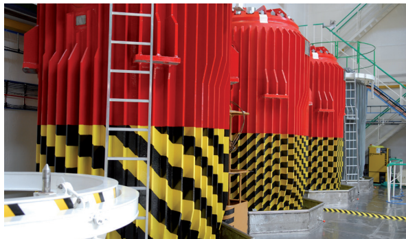
Transport containers for the shipment of spent fuel. Nuclear Regulatory Authority (NRA)
