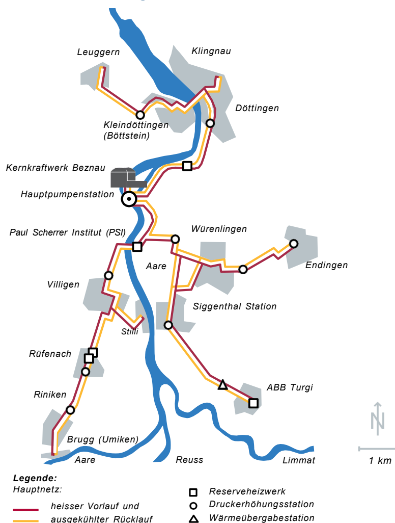
Figure 6.16: District heating network at the Beznau Nuclear Power Plant
