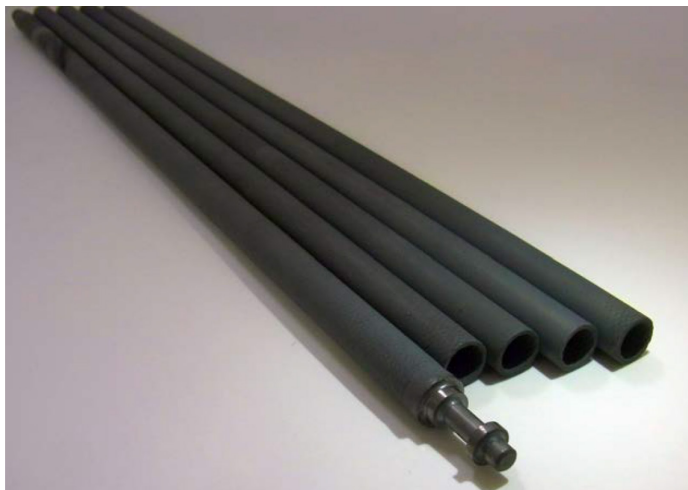
Figure 4-1: Cladding tubes made of a composite of SiC fibres and SiC matrix
