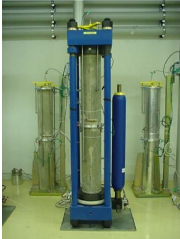
Figure 15. View of creep test on VeRCoRs concrete
