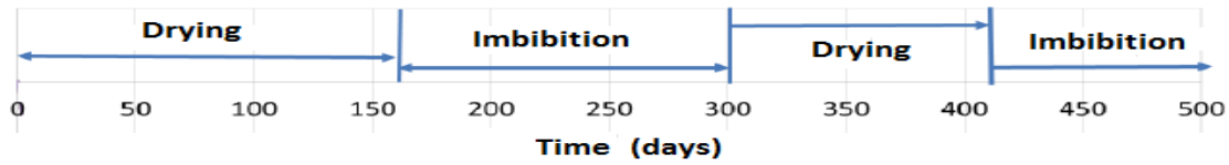
Figure 25. Programme of drying-imbibition cycles during the creep test
