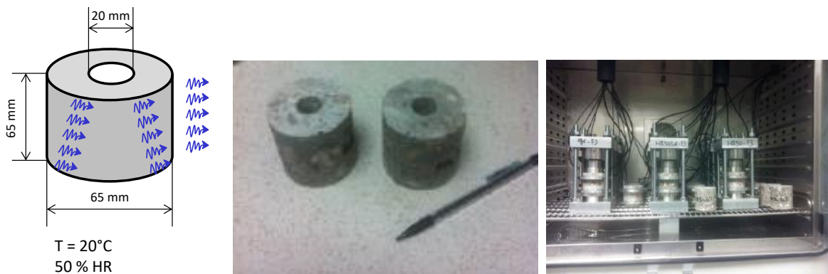
Figure 24. Views of drying-imbibition creep tests on hollow cylindrical specimens
