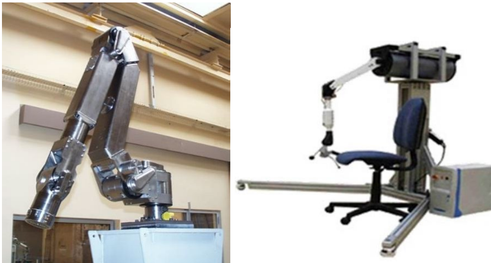
Figure B.8. The MAESTRO telerobot: Left, MAESTRO Slave arm; Right, MAT6D Master arm (EPRI, 2016)
