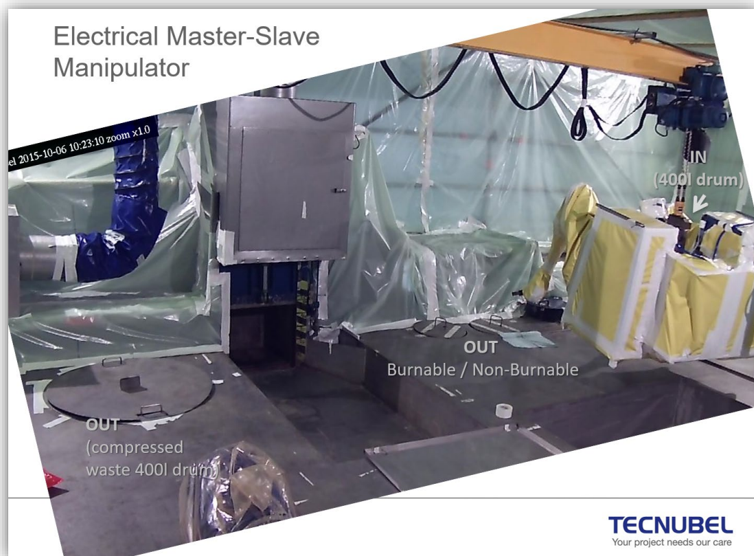
Figure B.28. EMS, wrapped in yellow foil, on mobile bridge above the working platform in a double tent confinement, equipped with a 100 tonne press (photo ENGIE Tihange Nuclear Power Plant )
