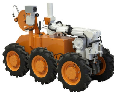
Figure B.27. Emergency response robot
