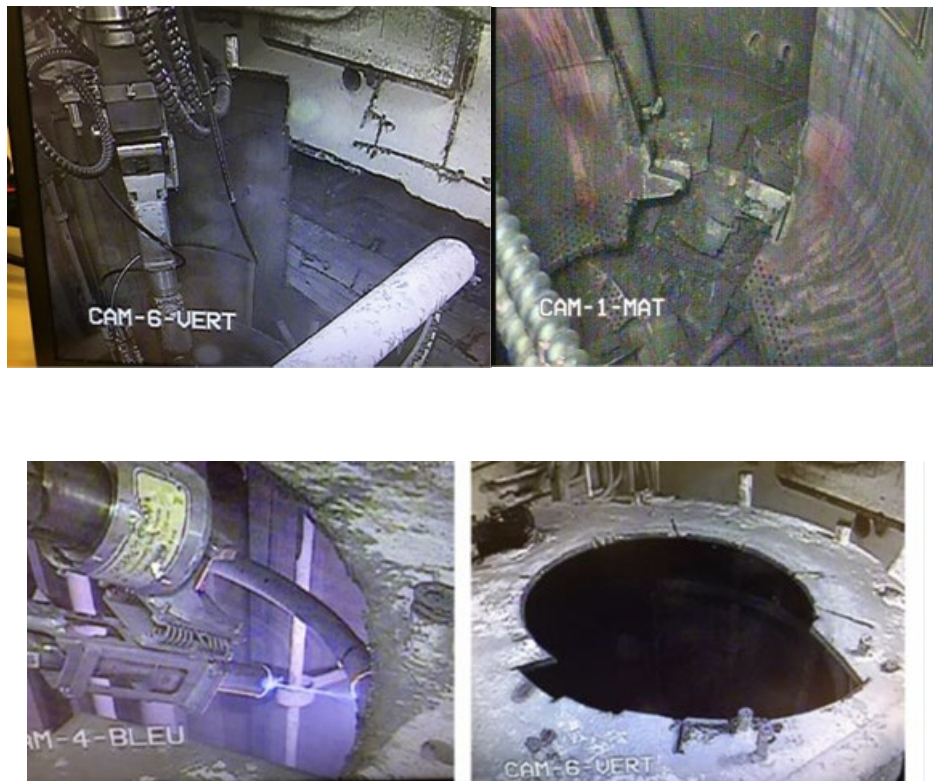
Figure B.10. MAESTRO in dissolver A of the Plutonium Plant n°1 of Marcoule
