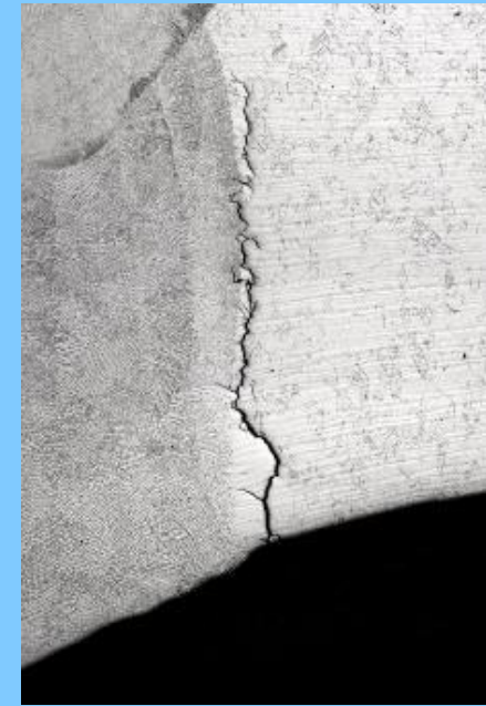
Crack propagation along grain boundary in heat affected zone of the weld
